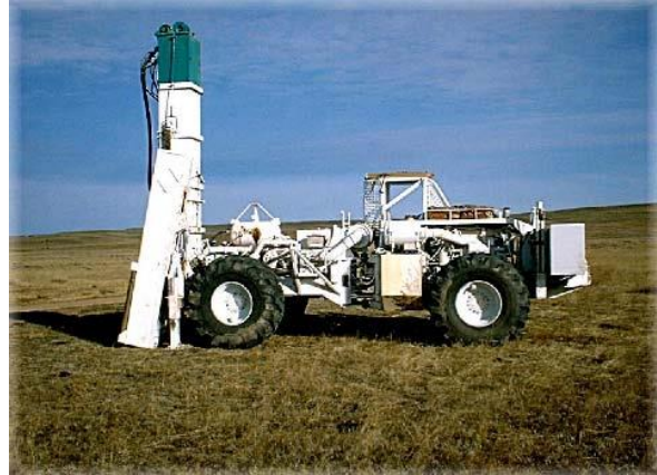
Photo 4 Buggy mounted drill. Photo: Duchesne Ranger District.
