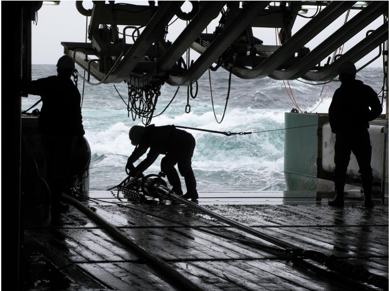
Photo 7 Silhouettes of persons recovering source (gun) array on seismic survey vessel. Sources are used to produce underwater acoustic sound waves with high pressure air. Jouni Niskakoski on Shutterstock.com
