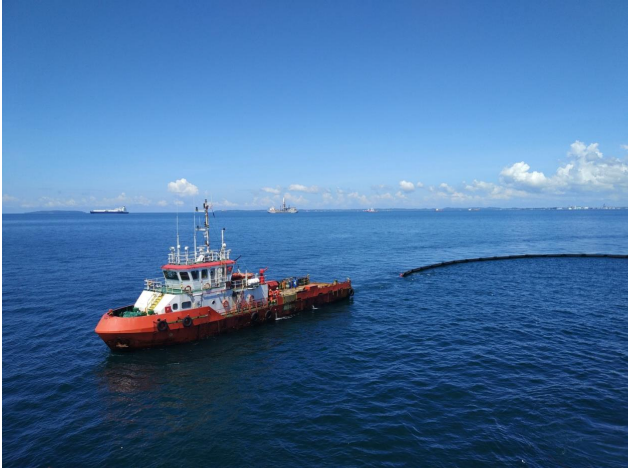
Photo 17 An offshore vessel performing oil spill response exercise in the middle of the sea. Oil spill response comprises of mother boat and a tow boat to carry oil spill boom. Mark_vyz on Shutterstock.com
