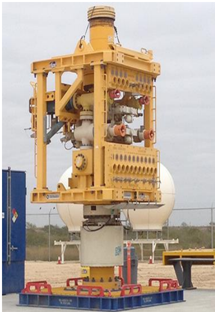
Photo 18 Capping stack image from NOAA at https://response.restoration.noaa.gov/scientific-support-coordinators-tour-deepwater-well-containment-facility
