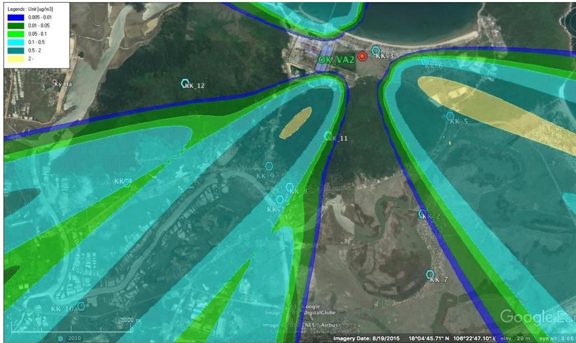
**Figure 3. 5- Annual PM<sub>10</sub> concentrations in the scenario of normal operation of VA2 Plant.**
